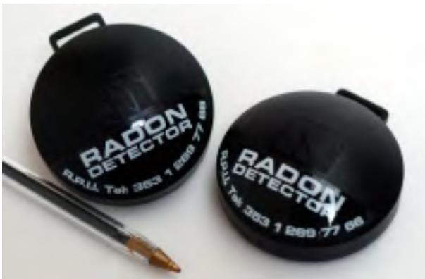
To the left is a modern nuclear track detector.
